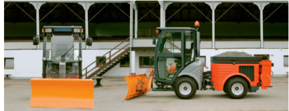
Citytrac Snow plough and gritting: Snow clearance with spring-mounted blade, 1.50 and 1.70 m, in combination with hydraulic rollers or combination gritting, 1.20 / 6 m working width
