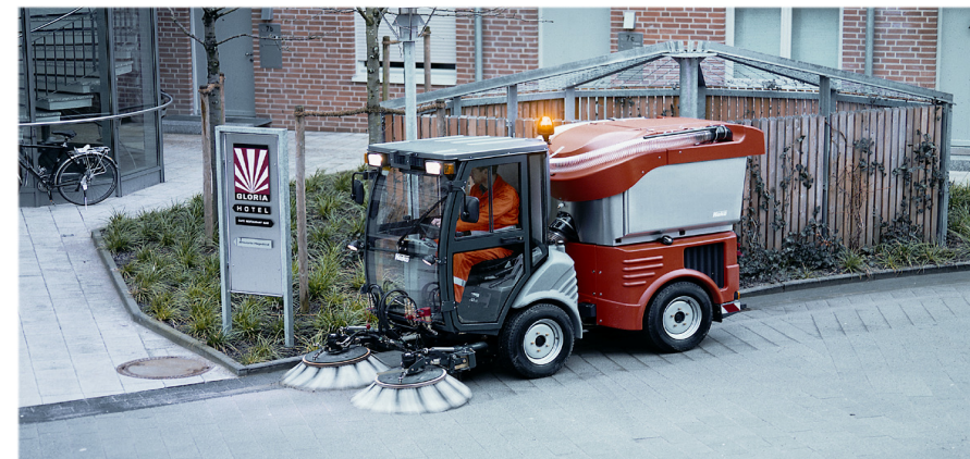
Citymaster Sweeping: Hydraulically powered suction fan
