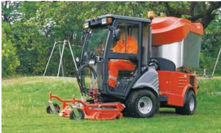
Citytrac Grass-Leaf vacuumunit In combination with lawnmower to collect directly the grass and leafes. The suction fan is hydraulically driven
